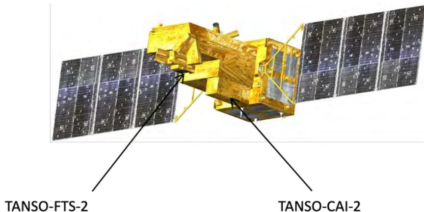
Fig. 1.3.1-1. Satellite image of GOSAT-2 and its two instruments
